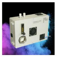
The test gas conditioning system GO-MO 3 comes with a permeation dryer and a test gas pump.
